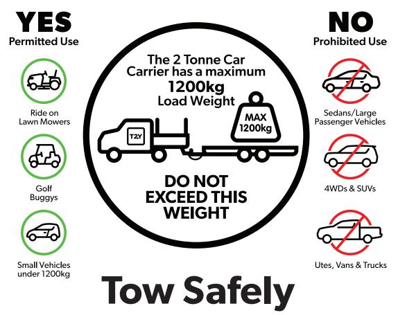
Stay Safe. It is the hirer's responsibility to check the weight of any vehicle being loaded onto a T2Y Car Carrier
